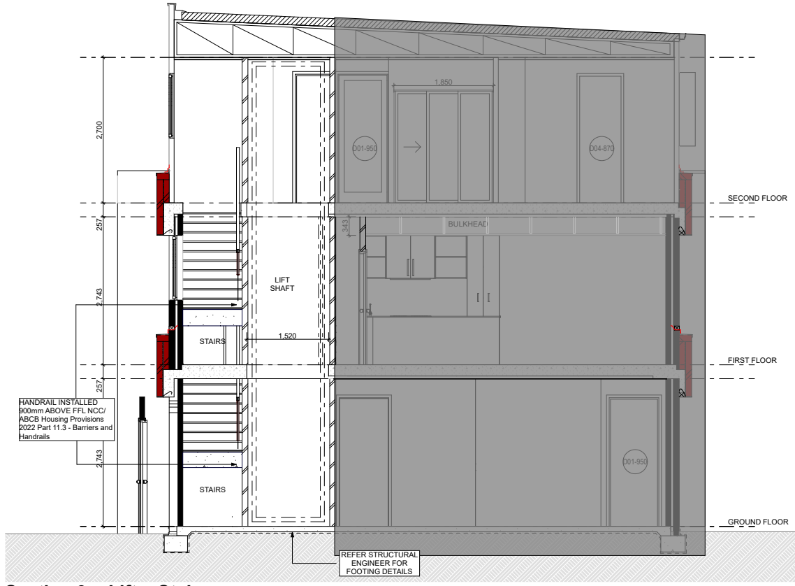
Section 3 - Lift + Stairs Scale 1:50
