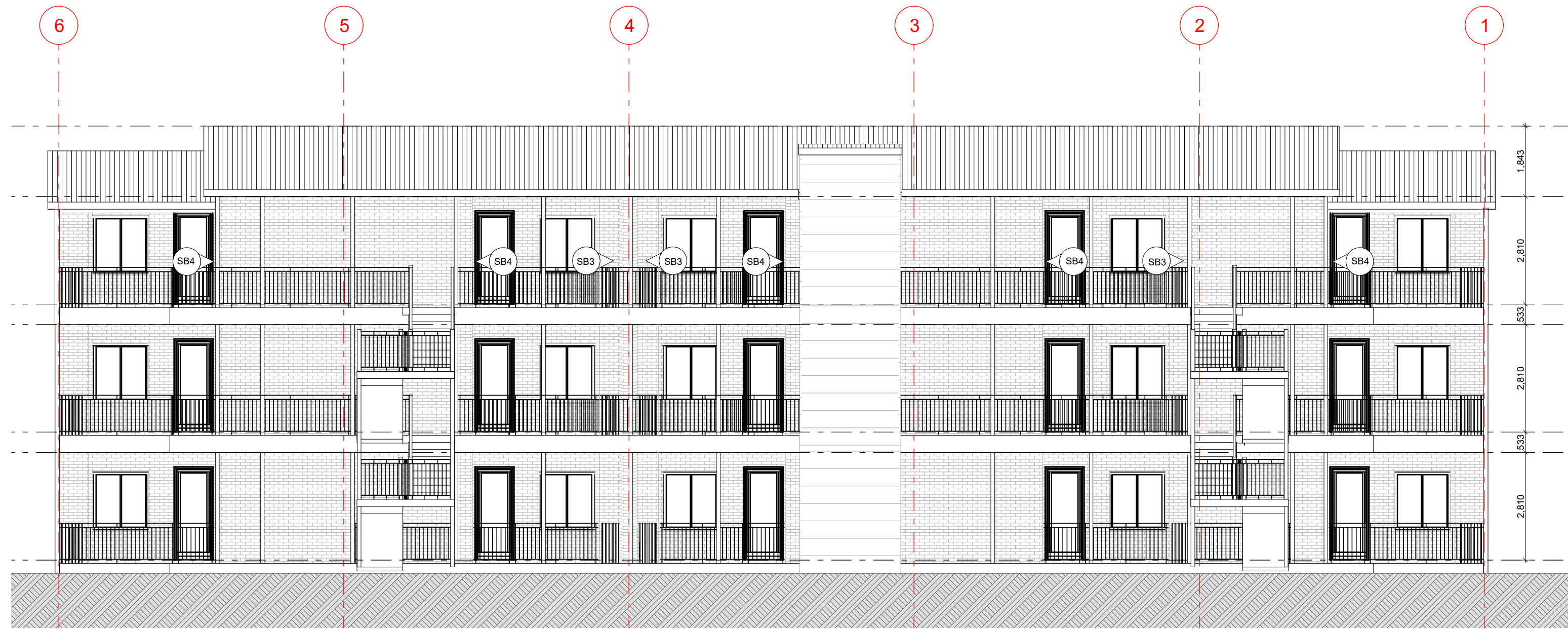
FRONT ELEVATION FACADE Scale 1:100
